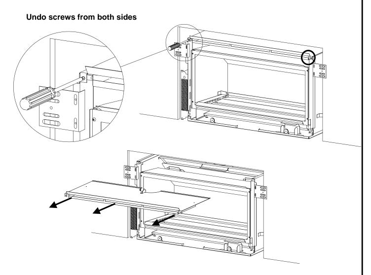
**Step 3:** For best access we recommend removing the fire box. Undo the four screws on the front four corners of the fire box and the two screws on the inside holding down the fire box (as shown below). Pull the fire box out of the heater.
