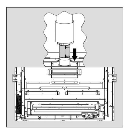
Once the gas fireplace has been inserted into the OSK and the firebox removed, the flue can be attached. To do this line up the 100mm flue with the flue outlet spigot and drop the flue into the spigot.
