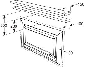
Maintain a 30mm clearance around the fascia to ensure ease of fascia removal.
