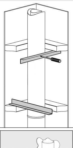
A length of angle should be attached to the inside of the timber frame cavity to hold the flue in place. Once you have fixed the angle to the inside of the cavity holes must be drilled to secure it to the flue. Screws or rivets can be inserted directly into the 150mm flue to hold it in place.
