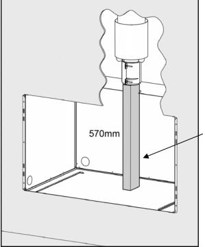
To make sure the flue is installed at the correct height, a piece of timber can be cut to 570mm and between the fire base level and the bottom of the flue. This will ensure the correct height for installation and support the flue assembly.
