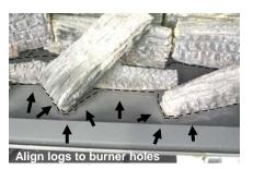
4) Cover empty spaces around logs on the front burner ONLY with small coals as provided. It is important that coals are not placed on the rear burner at all.
