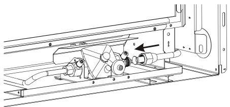
right. Each is sealed by a 'knock-out'. Remove only the knock-out which you require, and place the supplied rubber plug into the hole. You will need to make a small cut into the rubber plug to allow the gas pipe to pass through, keeping the plug as air-tight as possible.
