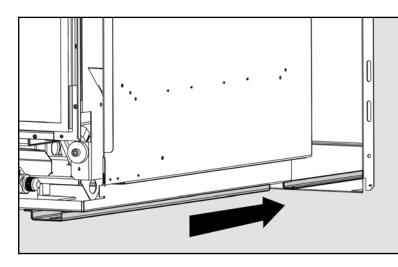
Attached to the base of the Outer Skin Kit are guide rails. The inside edge of these rails will line up with the outside edge of the two outer under base supports. When the parts are lined up, push the fire towards the back of the Outer Skin Kit until it cannot be pushed back any further. The front of the firebox should now be sitting flush with the OSK.
